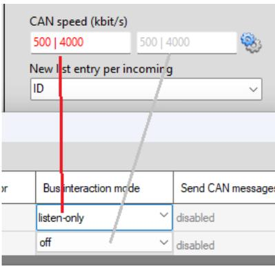
4. Choose to enable or disable message sending from the drop-down menu. This allows the user to lock out or enable each CAN channel from being able to send messages or not. If these are disabled, the Send CAN Messages Tab will not be functional
