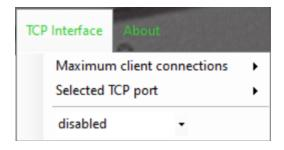
TCP/IP can support multiple connections so the user may specify the maximum number of connections are allowed to be accepted to the software. If the number is increased, the server opens the given number of network ports, starting from the port that gets defined. It is possible to open and stay connected simultaneously on different ports.
