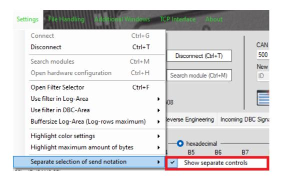
This menu item only impacts the Send Messages area. This allows the user to specify if they want to use separate send notations from the mean CAN ID dispaly format. Note that using the separate send notification allows the user to specify either Decimal or Hexadecimal in the Send message formatting.
