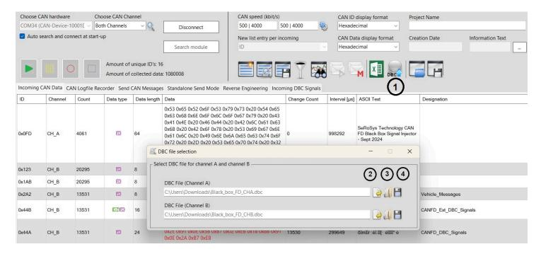
1. Press this button to open a dialog box to select a unique DBC file to load into each channel independently. The user may also edit the DBC messages and save DBC files.
