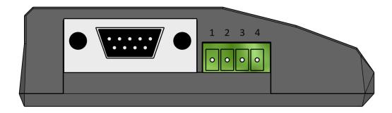
GPIO pins 1 and 2 are inputs
