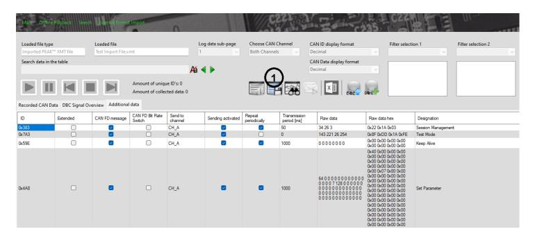
Step 3 (option 1) - To save it as a file to be able to be loaded into SLSS CANAnalyser main program Send CAN Messages tab, select the .CASF format option as the **Save as type** and then choose a file name
