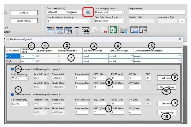
Press the image of the gears to open the Hardware Configuration window. The Connection Speed and Connection Mode for each channel can be adjusted here.
