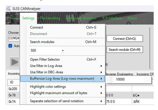
Going into this menu allows you to increase the maximum recording log buffer size. Note that the larger the log buffer, the longer it takes to save the exported data. A value entered higher than the allowed maximum will default to the maximum value.
